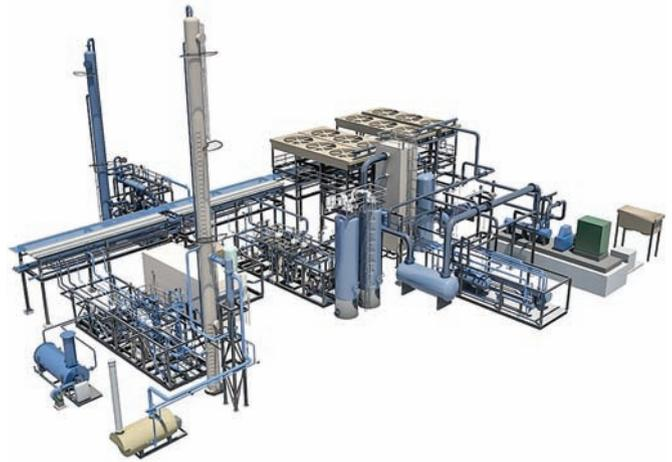
**FIG. 10.** Schematic of a preengineered modular plant.
