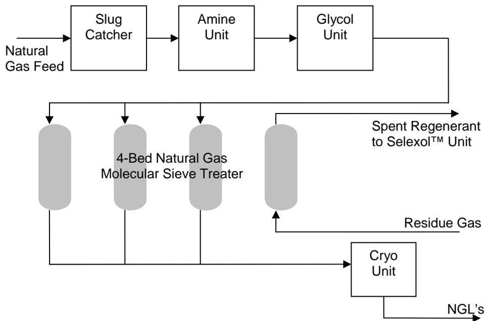
Figure 1 – Simplified Block Flow Diagram
