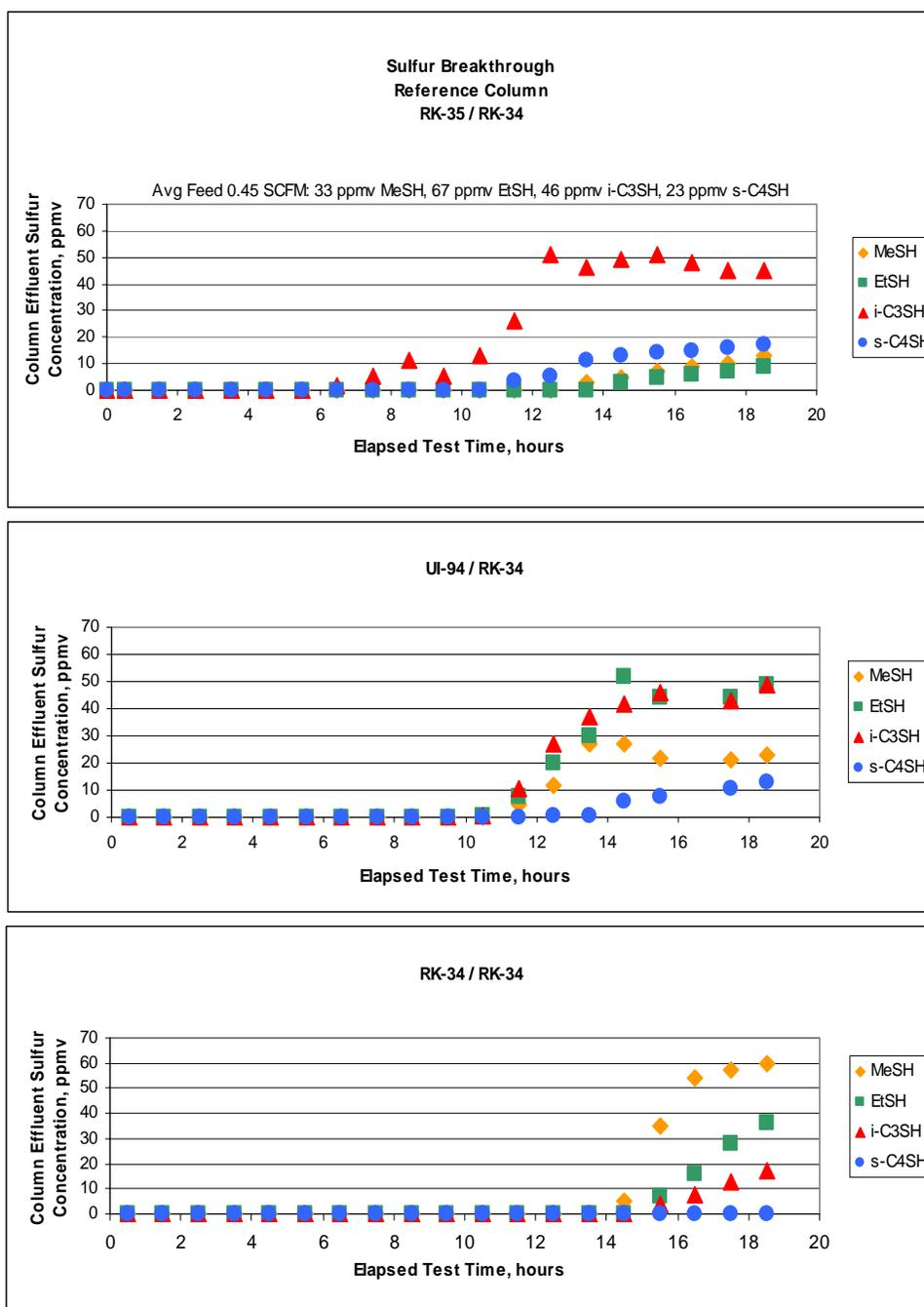
Figure 6 - Aged Adsorbent Sulfur Capacity Evaluation
