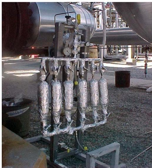
Figure 4 - Product Aging Test Rig
