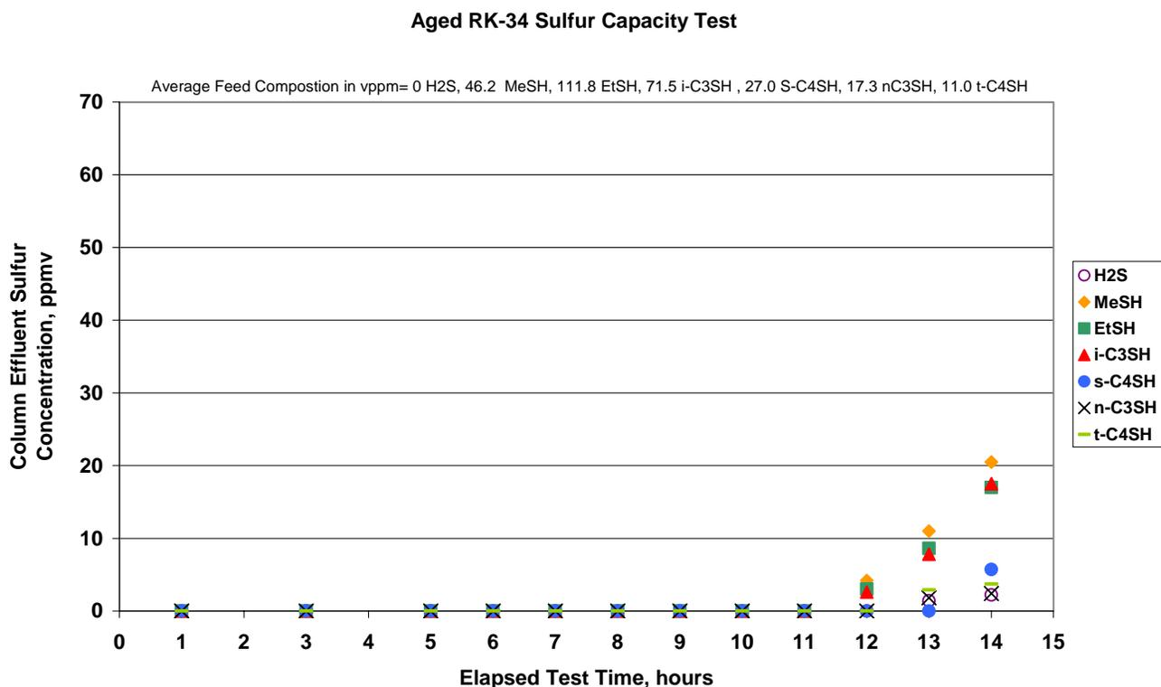
Figure 7 - Aged RK-34 Adsorbent Sulfur Capacity Test
