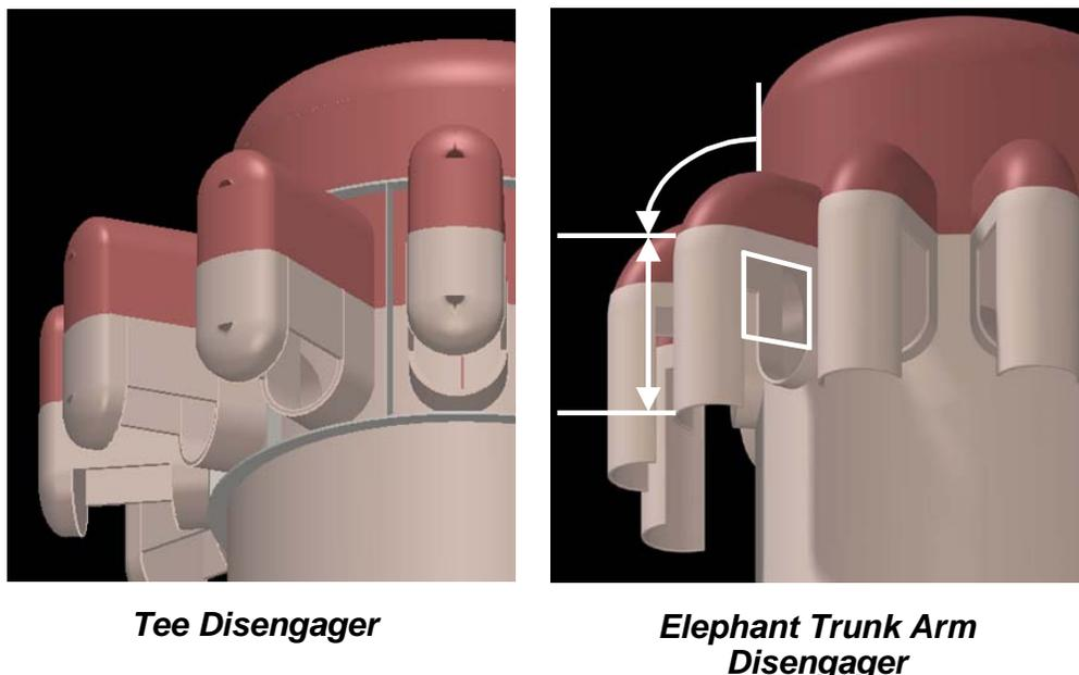
The CFD model of the final design indicated that at a superficial velocity of 1.05 m/s, slightly higher than the base case model, the gas velocities exiting the arms of the elephant trunk disengager were significantly lower than the gas velocities for the tee disengager with peak gas velocities reduced by 25% and the horizontal gas velocities at the dipleg outlets reduced to nearly zero; see Figure 10.
