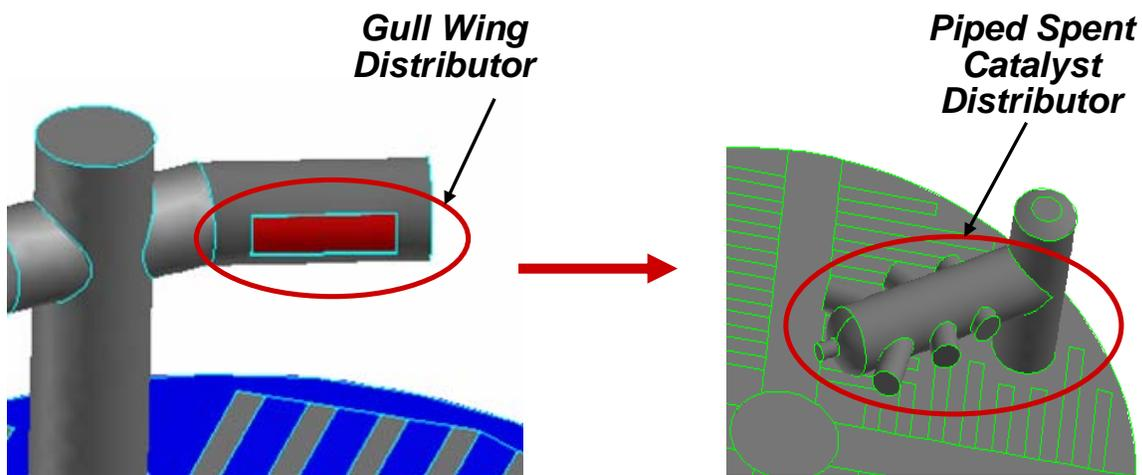
CFD models of the gull wing distributor and the piped spent catalyst distributor were created to predict the catalyst distribution, gas flow paths and bed density profiles in the bubbling bed regenerator. With the gull wing distributor, the catalyst was concentrated in the center of the bed. With the piped spent catalyst distributor, the catalyst distribution was much more uniform throughout the bed; see Figure 13.
