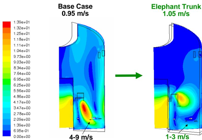
With the original design, ten out of eleven inner cyclones holed-through after six years of operation. With the installation of the elephant trunk disengager, the fines entrained to the inner cyclone set were reduced sufficiently to reasonably expect a 10 year service life. This enables the refiner to either significantly reduce maintenance costs and realize greater on-stream reliability, or to push the system harder for greater operating margin.
