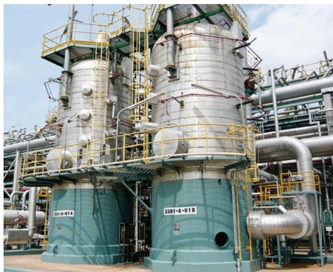
**FIG. 4** Parallel fixed-bed reactors using advanced adsorbents at the PTT GSP-5 gas plant, Map Ta Phut, Rayong, Thailand.
